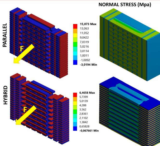
**FEM simulation** A FEM simulation was performed using ANSYS. The simulation replicated the tensile test executed on the 3d printed specimen. The material was allocated based on the machine path during the manufacturing. To simplify the model, a depth equal two times the hatching is assumed. Due to the non-axial symmetry, it was necessary to use the entire cross section of the specimen. Here are some parameters of the simulation:
