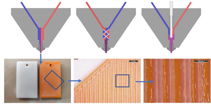
On top from left to right: (1) Coextrusion; (2) Interlocking; (3) Blending
